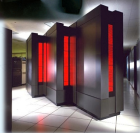
The CM-5 is MIMD (Multiple Instructions Multiple Data) using commodity SPARC processors using a "fat tree" interconnect
